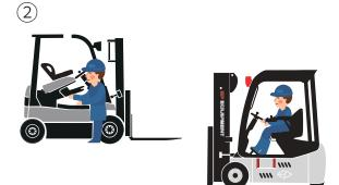
Lift up the driver seat and disconnect the battery.
